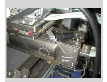
1. Remove Vision X-Axis motor from the gear rack interface only.
