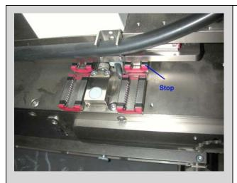
3. Standing behind the machine slide the vision system to the left, just enough to expose the sensor.
